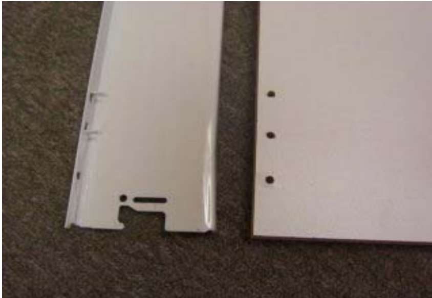
Both prongs are inserted into the back holes and the front hole will be for a euro screw to hold the bottom in place
