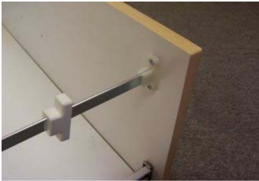
Insert side file bar into bracket on back of front
