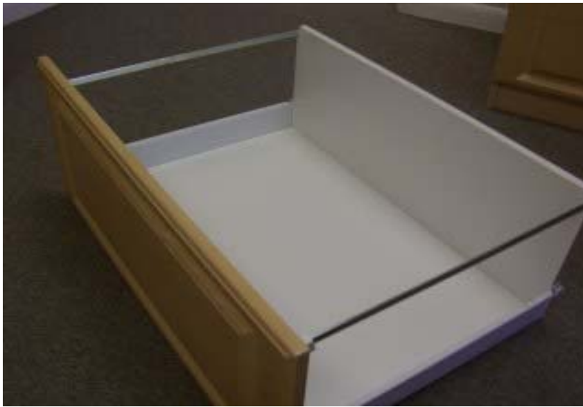
Drawer Box Assembly is complete and now ready for Lat bars.
