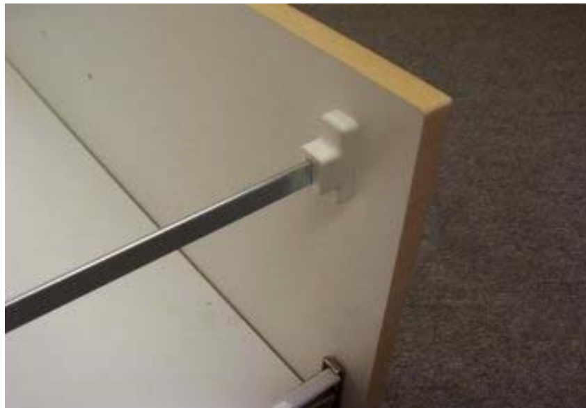
Slide bracket cover over bracket after bar is inserted.
