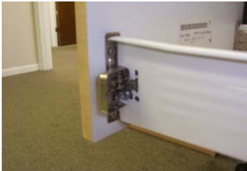
Place front onto drawer box assembly with clip in the open position.
